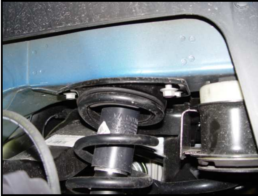
Figure 4 - Four upper strut mount bolts
